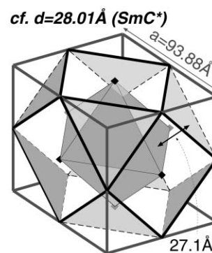
Fig. 4 Cubic I432 structure of IsoX in ( R,S )-FPPY determined by X-ray diffraction. This figure was quite simply drawn, and it is considered that it would actually relax to the Schwarz P surface structure as shown in Fig. 6 of ref. 9.
